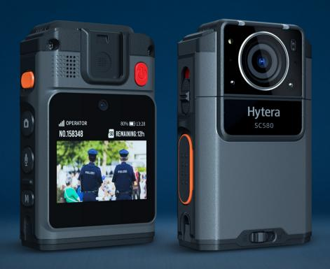
Hytera SC580 smart 4G body camera captures high quality videos, audios, and photos and stores them securely. When the situation requires it, the body camera can transmit and livestream video from the field to the command center over the cellular network or WLAN.
